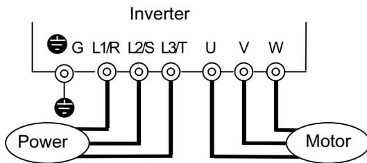
Figure 3-1-1 Inverter connection
